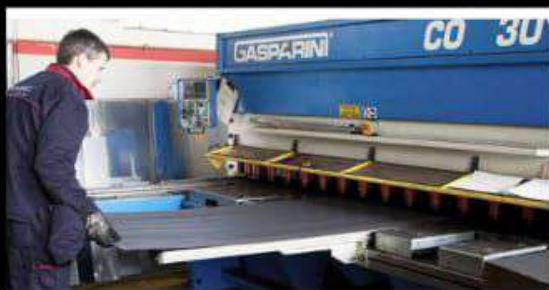
MS sheet sharing (cutting) process
