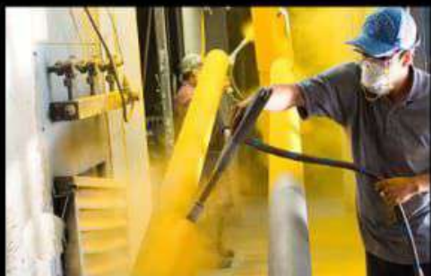
powder coating with chemical treatment
